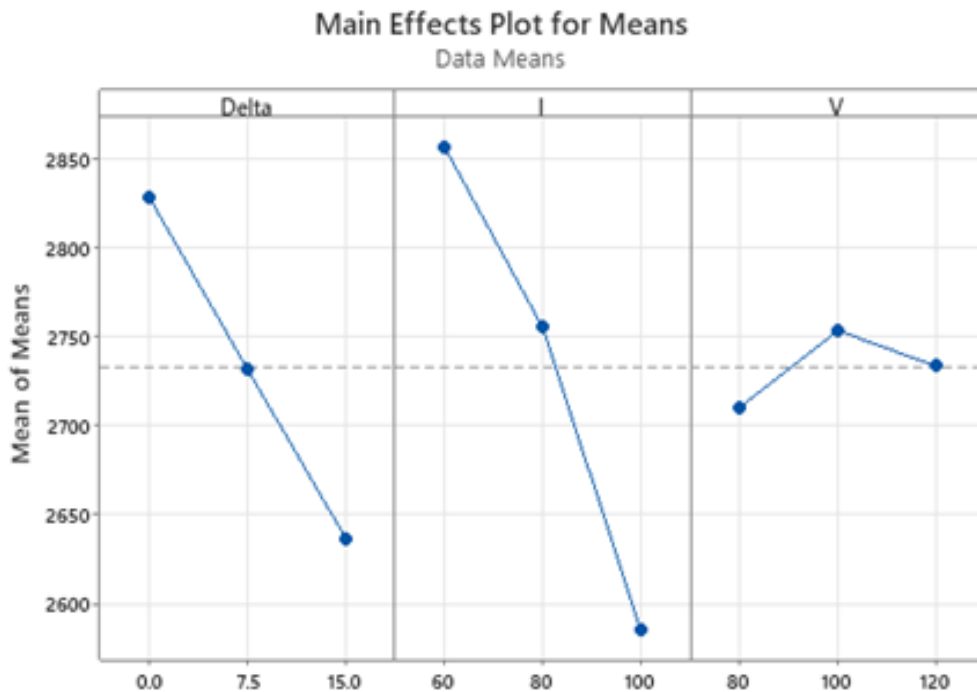
Fig. 2. Main effects plot for mean hardness
